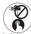
Don't pull wire to unplug machine, switch off & catch the plug and pull out.
